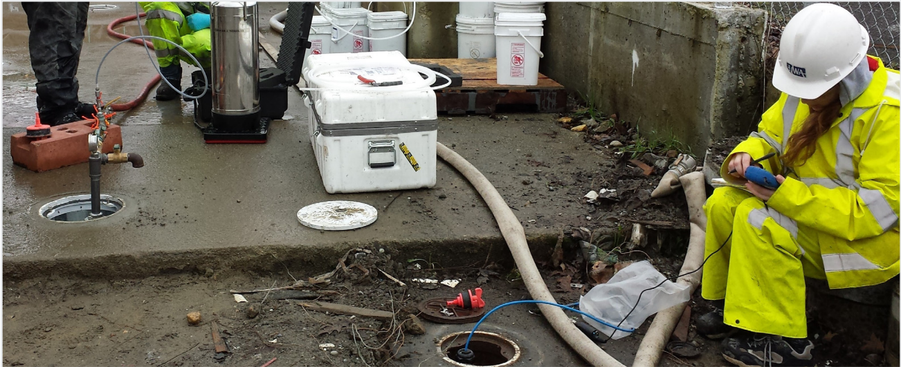
Trace testing using the In-Situ TROLL 9500 Multiparameter Sonde and RuggedReader Handheld PC. Photo courtesy of HWA GeoSciences Inc.
